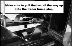
Check that the box is securely on the trailer frame at the front and rear of the box.
