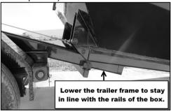
8. Make sure to pull the box all the way up onto the trailer frame stop before lowering the trailer frame onto the crossmembers of the trailer.
