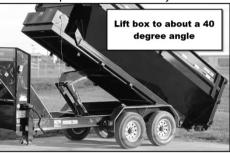
3. Start letting out the winch for the box to slide off slowly, if box does not begin to slide, raise the bed with the KTI hyd. unit a little more. Ensure the trailer rails don't dig into the ground.
