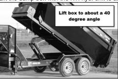
Start letting out the winch for the box to slide off until the back end hits the ground, if box does not begin to slide, raise the bed with the KTI hyd. unit a little more. Ensure the trailer rails don't dig into the ground.
